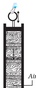
Fig. 15.4 Longitudinal waves (sound) generated in a pipe filled with air by moving the piston up and down. A volume element of air oscillates in the direction parallel to the direction of wave propagation.
