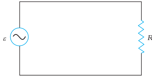
FIGURE 7.1 AC voltage applied to a resistor.
